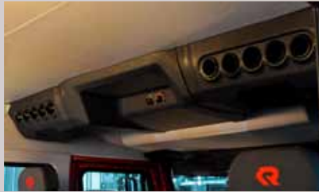
■ Dual outboard HVAC for crew
