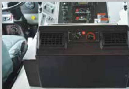
Engine Tunnel HVAC
