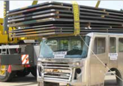
120,000 lb. Crush Test
